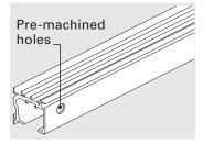
Screw fix the track to the stud wall using #8 screws, ensuring it is level and solid enough to support the door weight.
