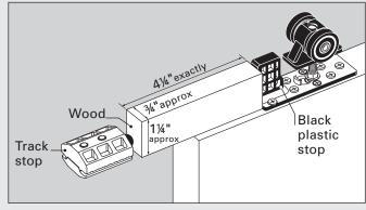
d) If you have a twin mechanism (soft close & soft open), you will need two activators. Repeat the steps above for the other end.
