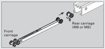
Make sure the front carriage with the tow bar connected to the soft close mechanism faces the end of the track that you want to soft close.
