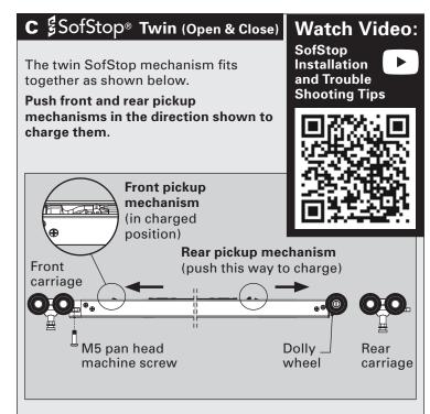
Most of the time you will have the room to slide the mechanism in from the end of the track fully assembled.
